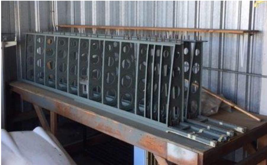
Here's a picture of the wing spars, main ribs, and rear spar. Nose ribs are primed and prepped also. I removed them from the jigs. Next picture is of the empennage. It has electric rudder trim.
