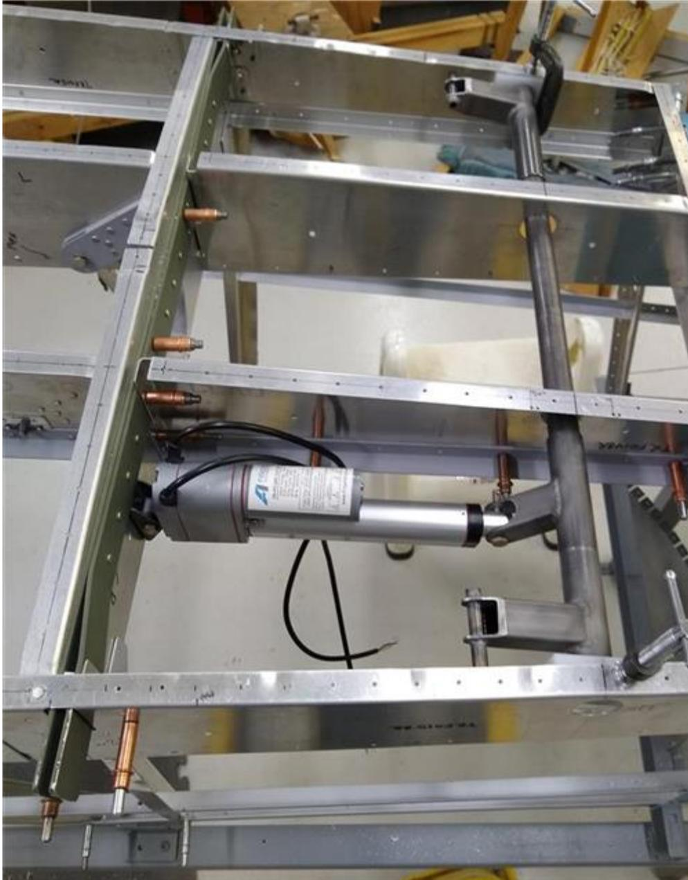
We're working on a new, completely **beneath the floor, flap drive mechanism**. We can't claim this idea. It came from Paul Romano, with help from Ray Ward.
