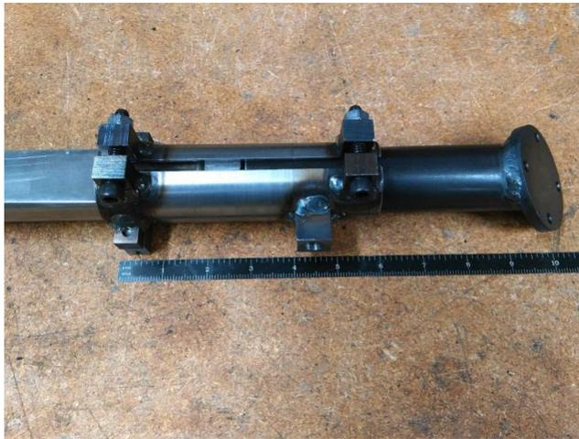
*Gear leg clamps:* Setting the wheel alignment can be difficult. We recently designed, and are now producing, a gear leg/axle socket clamp that should allow the alignment task to be delayed until the plane is nearly finished, when it will be at a proper weight to set the wheel alignment. I won't go into details here, but we think this is a cool idea that solves a real problem.
