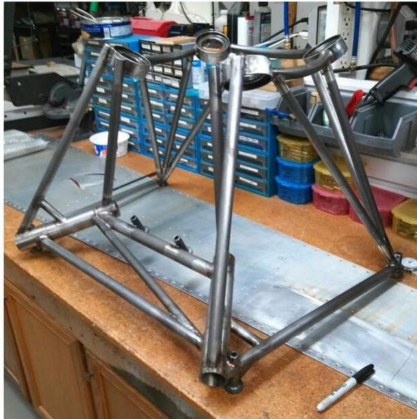
With Aircorps Aviation handling the sheet metal, it was time to find someone to help with the engine mount that we needed. I was still at Oshkosh 2016 at this time, so it didn't take long to find the Javron display. They were obviously steel tubing experts. Soon, they were making some gorgeous engine mounts just for the 4 cylinder F4s. Nice!
